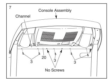
8. Hand tighten four additional Screws (3) into the Handrail (20) and the console assembly. Then, tighten all nine Screws used in step 7 and this step; do not overtighten the Screws.
